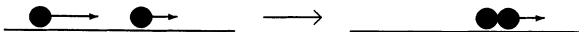
FIG. 1. Schematic illustration of the irreversible traffic model. A faster car overtakes a slower car and after the encounter the faster car assumes the velocity of the slower car.
